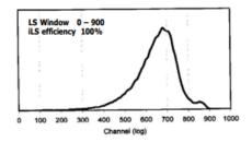
Crystal scintillation well counting. Thick (1" x 1") crystal scintillation detector. GM efficiency (4 $\pi$  at 1 cm) End window: 0.0%. Pancake: ~4%.
